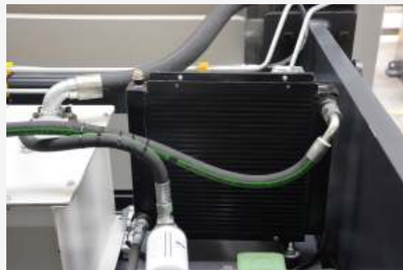
Hydraulic Oil Cooler System
