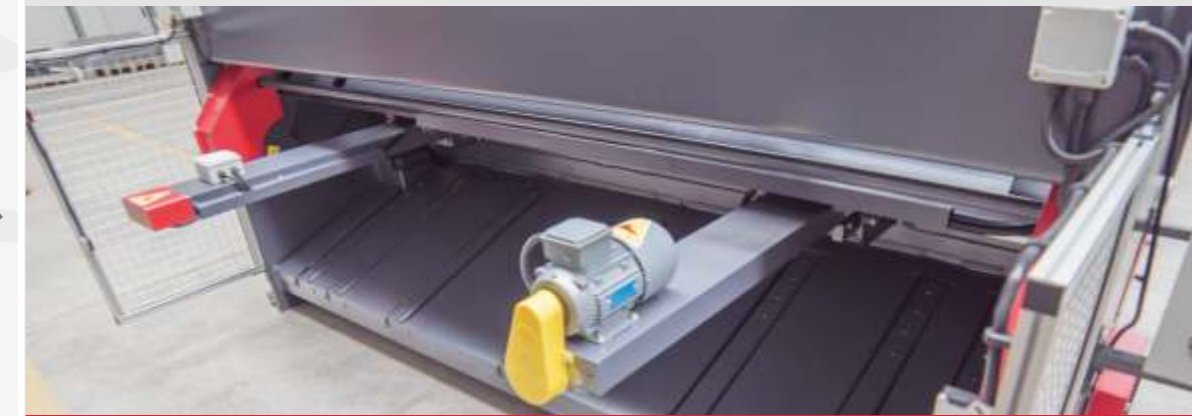
Motorized Back Gauge has \pm 0,1 mm Accuracy
